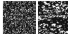
The uniform distribution of smaller spherical carbides in the powder metallurgical structure compared to conventional tool steels with large angular carbides and carbide clusters.
