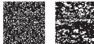
The uniform distribution of carbides in the powder-metallurgical structure compared to conventional tool steels with big carbides and carbide clusters.
