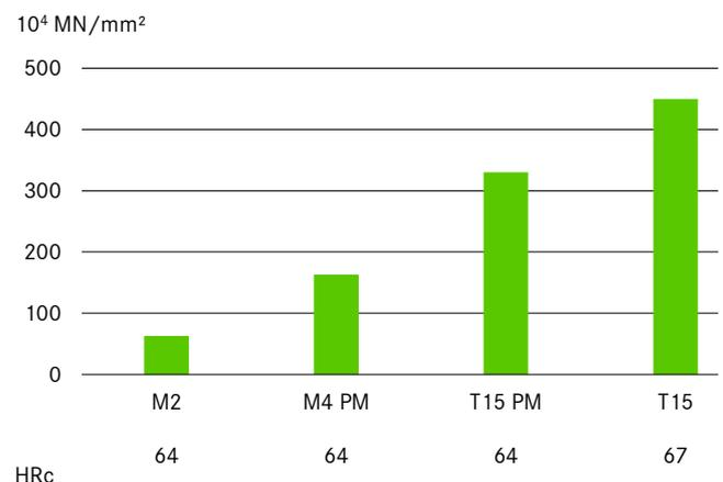
Reciprocal of wear rate in wear test with non lubricated crossed cylinder in contact with a rotation tungsten carbide cylinder.
