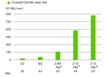
Reciprocal of wear rate in wear test with non lubricated crossed cylinder in contact with a rotation tungsten carbide cylinder.
