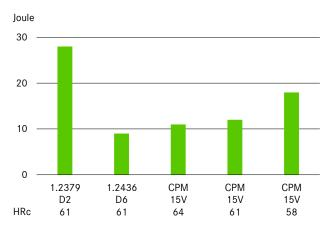
Standard size of the Charpy-test-piece with a 12.7 mm notch radius.
