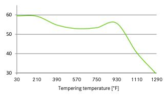
According to the required hardness and the actual dimension the hardening and tempering temperature have to be selected from the respective ranges.
