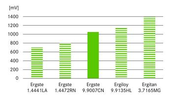
Corrosion resistance of  $\mathsf{Ergste}^{\circledast}$  9.9007 CN in comparison with other implantable materials.
