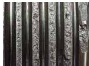
D2 Wear & Breakage
