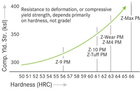
**Z-M4 PM®** — traditional PM grade for powder compaction applications offering a good combination of toughness, wear resistance and compressive strength.
