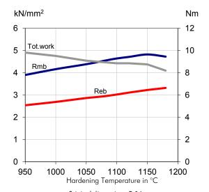
Original dimensions Ø 16 mm Tempering 3 x 1 hour at 560°C Dimensions of test piece Ø 4.7 mm
