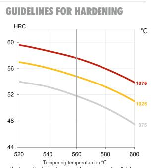
Hardness after hardening, quenching and tempering 3x1 hour
