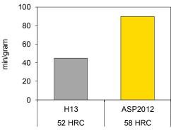
Wear resistance is measured as the time needed for removal of one-gram material from a test piece. Technique: Pin-on-cylinder, dry SiO2-paper of grade 00,
