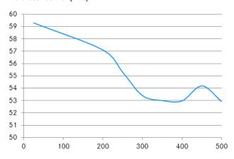
Tempering temperature in °C t= 30 min const.
